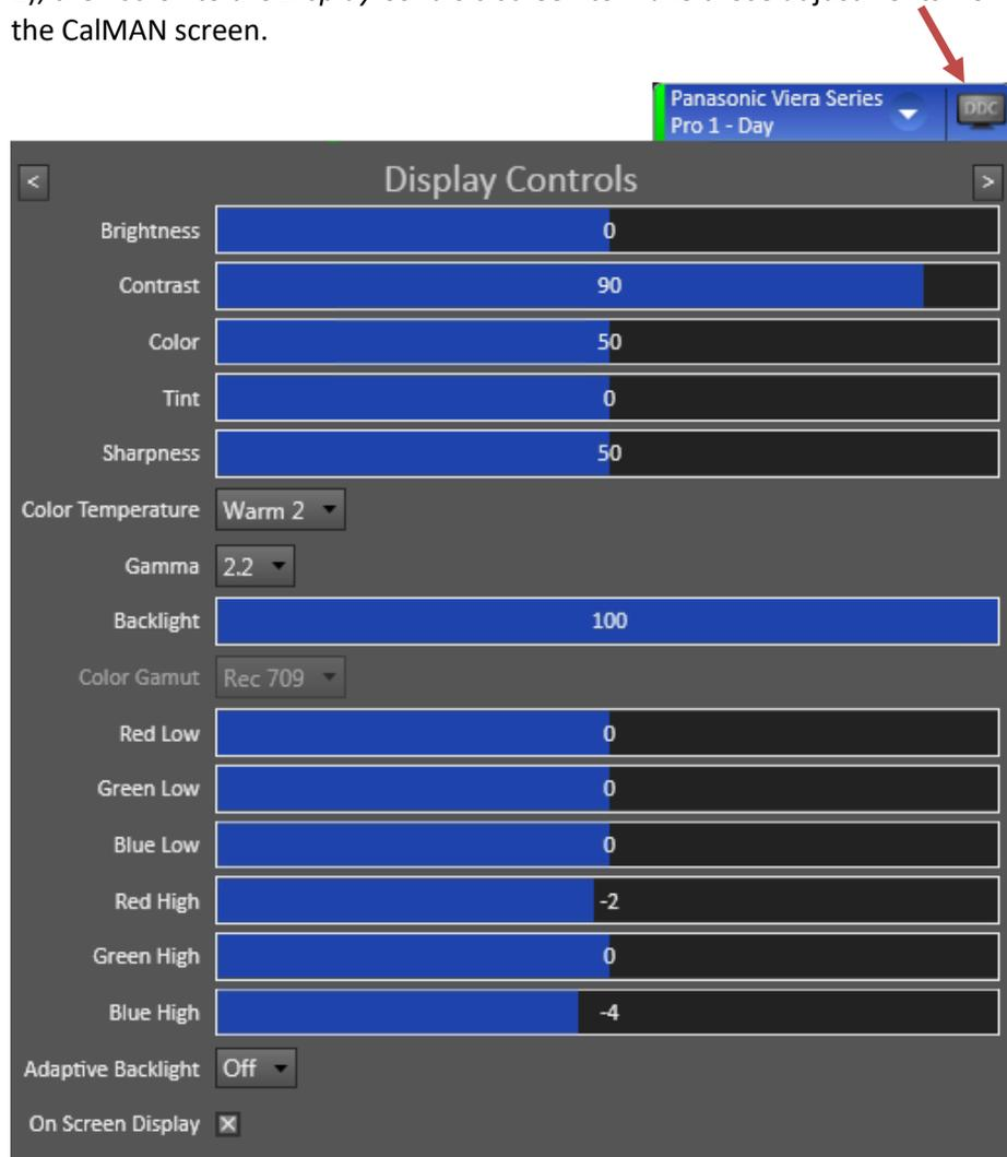
Figure 1. The display's picture controls can be manually adjusted directly from the CalMAN software, on the DDC Display Controls screen.
