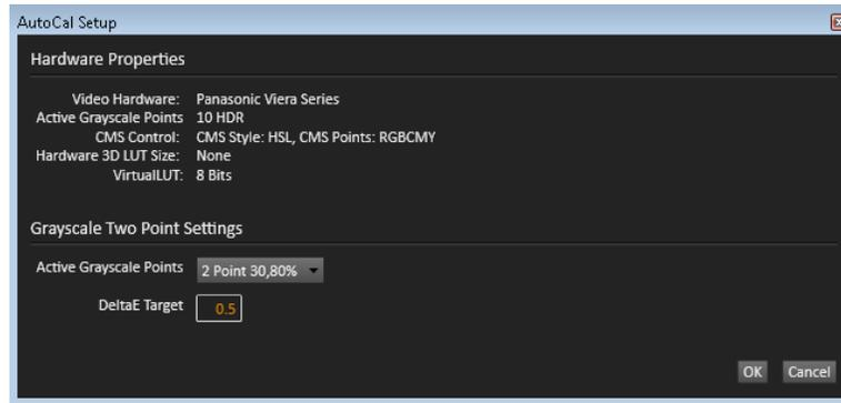
Figure 12. CalMAN AutoCal Setup dialog, for HDR10 White Balance calibration.
