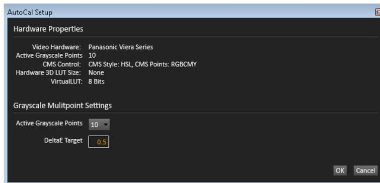
Figure 6. CalMAN AutoCal Setup dialog, for SDR Grayscale/Gamma calibration.
