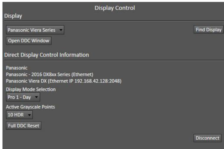
Figure 11. CalMAN Display Control tab, for selecting display control options.
