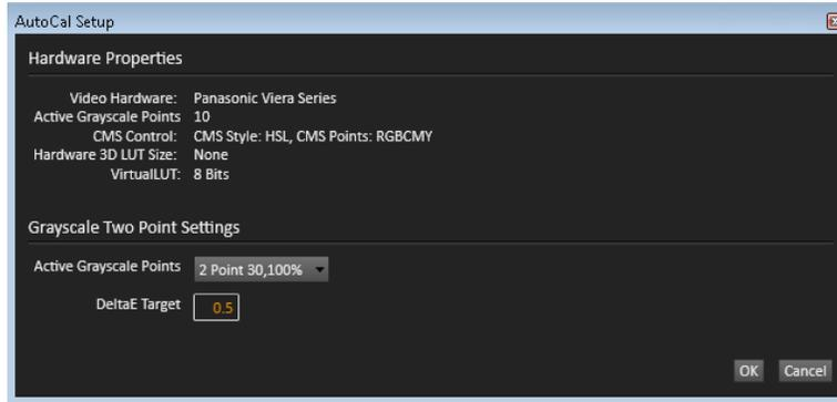
Figure 5. CalMAN AutoCal Setup dialog, for SDR Grayscale – 2pt calibration.
