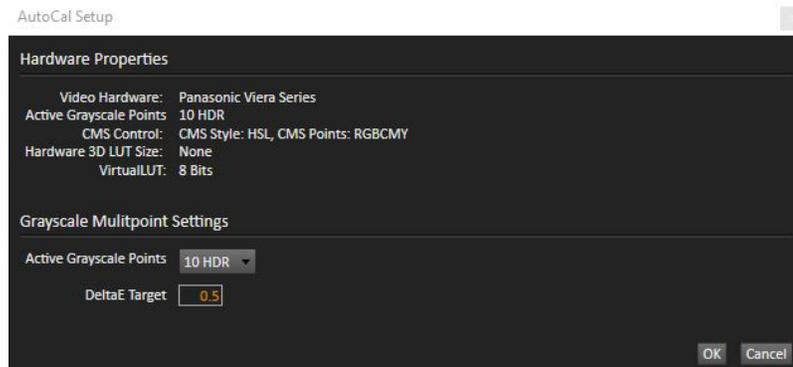
Figure 13. CalMAN AutoCal Setup dialog, for HDR10 Grayscale calibration.
