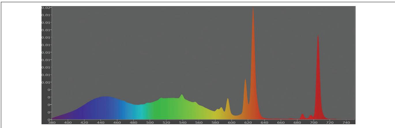
**Figure 2.** SPD of a typical CRT.
