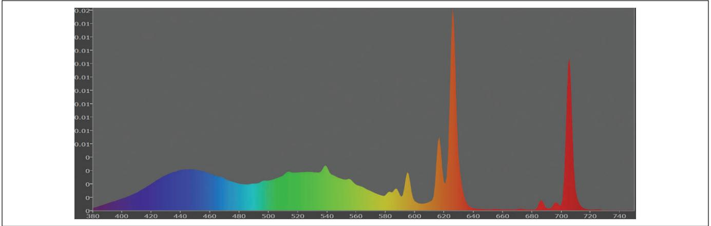
Figure 2. SPD of a typical CRT.
